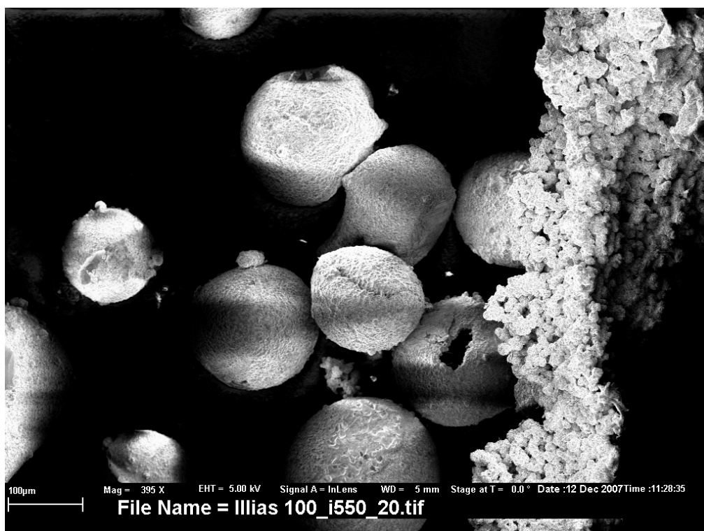
Fig. 7-17: Formation of Zn droplets and simultaneous oxidation at T=823\text{ K} , 100% \text{CO}_2
