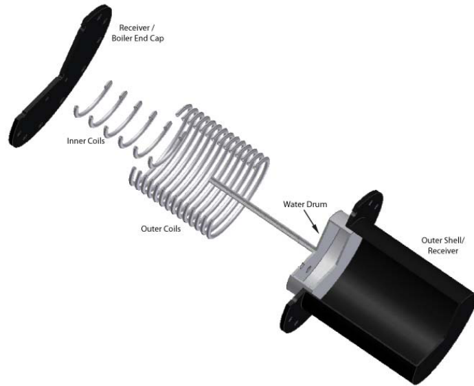
Figure 1.10: Receiver Assembly for Solar 1 [8]
