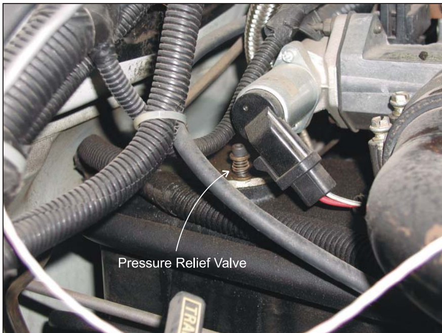
Figure 3-7 Pressure Relief Valve on Engine Crankcase
